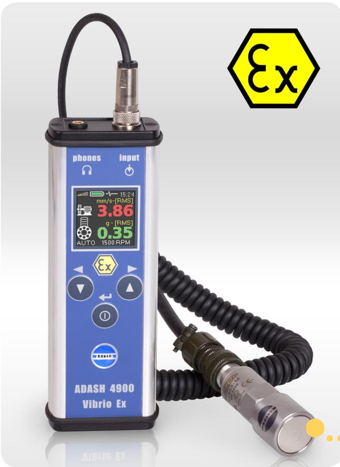
The A4900 - Vibrio M Ex instrument allows you to perform all basic vibro-diagnostics measurements such as bearing condition, identification of mechanical faults and lubrication assessment.
